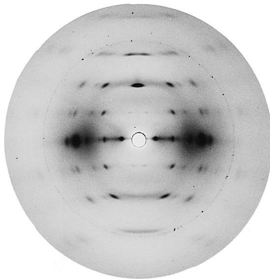
Fig. 1. X-Ray diffraction pattern from a polycrystalline and well oriented fiber of guaran (81% r.h.) which was tipped approximately 9^\circ towards the incident beam in order to register the meridional reflection on the second layer line.
